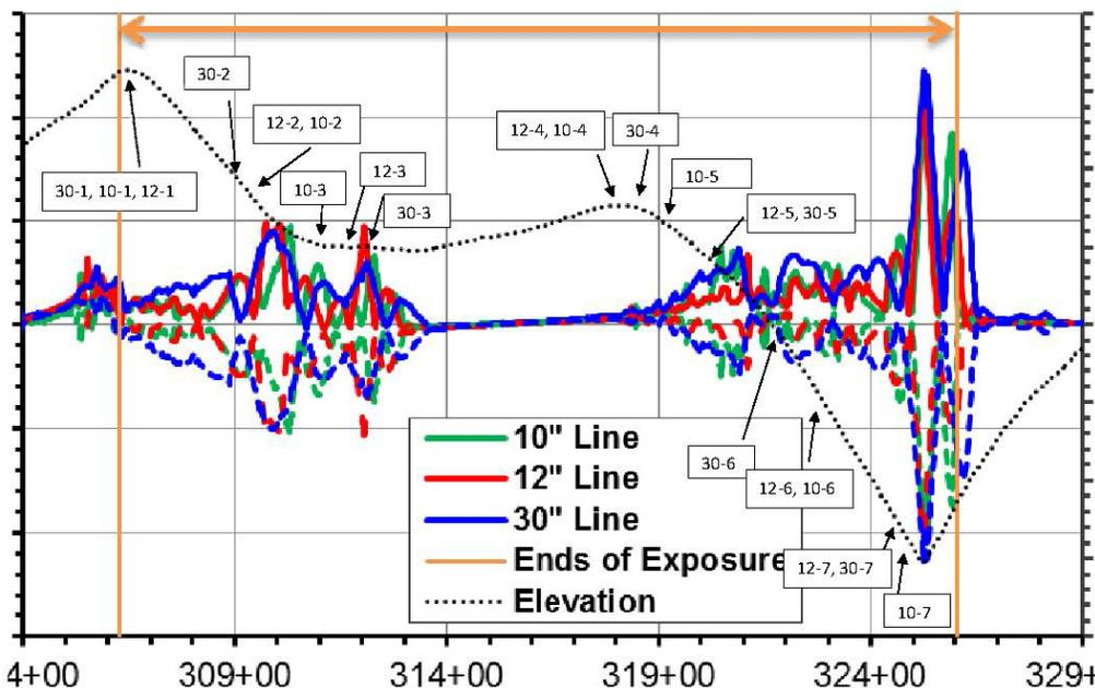
Figure 1: Gauge Locations, Stress Prediction, and Elevation Profile
