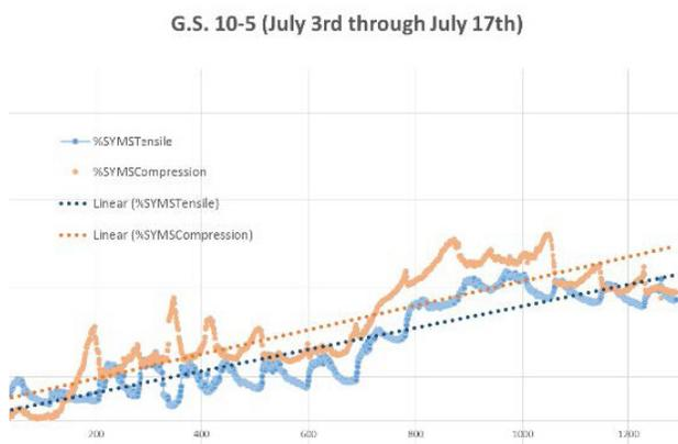
Figure 3: Trending Data of Pipeline Stress Over 2 Weeks
