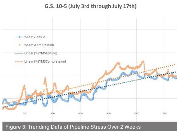
Figure 3: Trending Data of Pipeline Stress Over 2 Weeks
